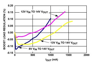
FIGURE 3. BOOST LOAD REGULATION @ 650kHz
