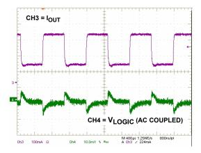
FIGURE 13. BUCK TRANSIENT RESPONSE @ 1.3MHz
