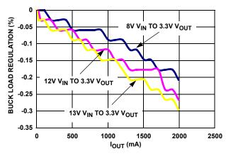
FIGURE 10. BUCK LOAD REGULATION @ 650kHz
