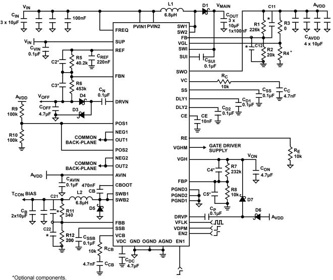
NOTE: Separate PGND and SGND planes must be used, see PCB layout procedure section.
