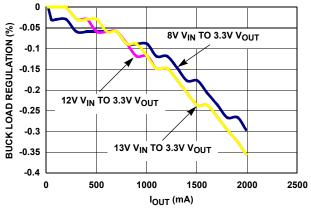
FIGURE 11. BUCK LOAD REGULATION @ 1.3MHz
