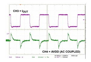
FIGURE 7. BOOST TRANSIENT RESPONSE @ 1.3MHz
