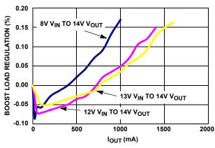
FIGURE 4. BOOST LOAD REGULATION @ 1.3MHz
