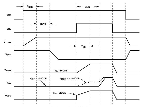
FIGURE 22. TIMING DIAGRAM 1
