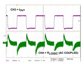
FIGURE 12. BUCK TRANSIENT RESPONSE @ 650kHz
