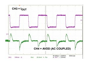
FIGURE 6. BOOST TRANSIENT RESPONSE @  $650 \mathrm{kHz}$
