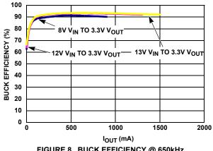
FIGURE 8. BUCK EFFICIENCY @ 650kHz
