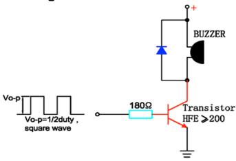
The base current Ib should high enough so that it saturates the collector current of the transistor with the CB load.
