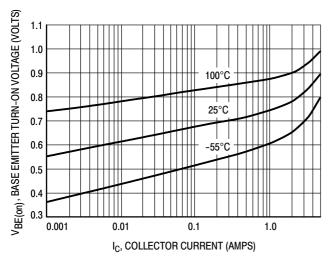
Figure 5. Base Emitter Turn-On Voltage versus Collector Current
