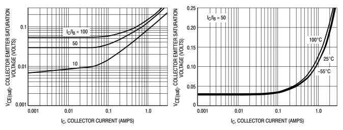
Figure 1. Collector Emitter Saturation Voltage versus Collector Current
