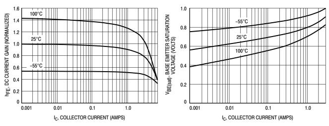
Figure 3. DC Current Gain versus Collector Current
