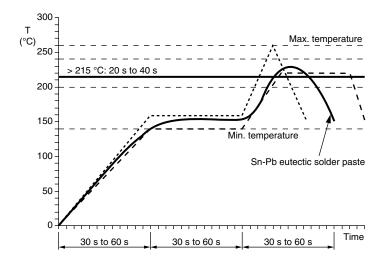
Fig. 6 - Soldering IR Reflow with SnPb Solder
