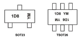
1D8 = Product Type Marking Code YM = Date Code Marking Y or  $\overline{Y}$  = Year (ex: C= 2015) M = Month (ex: 9 = September)
