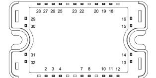
All multiple inputs and outputs must be shorted together Example: 13/14; 29/30; 22/23 ...
